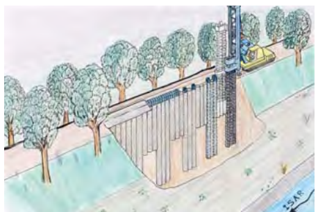
Hidden mixed-in-place wall
